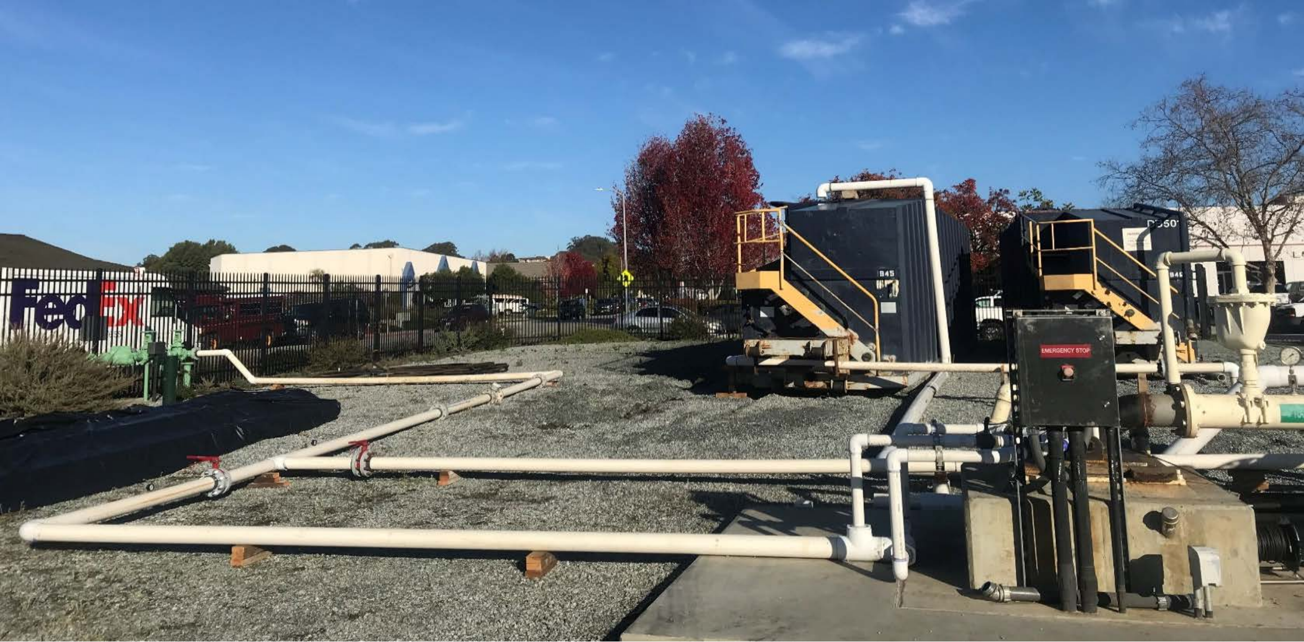
ASR Pilot Testing underway at Beltz 12. 22 MG injected and recovered (March, 2019)
