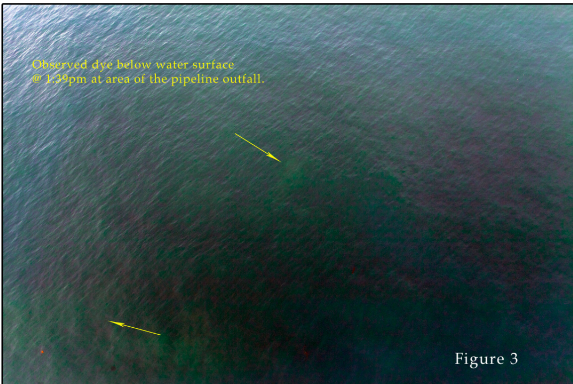
Figure 3 - At 1:44 the dye is observed below the water surface at the pipeline outfall. Continuous flight lines were flown along the entire length of the pipeline from the vault to the outfall and no other dye was observed.
