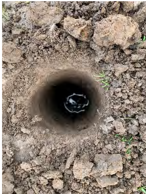
Example of Borehole showing shallow groundwater
