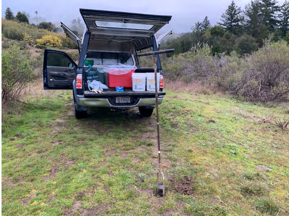
Hand Auger used to collect samples
