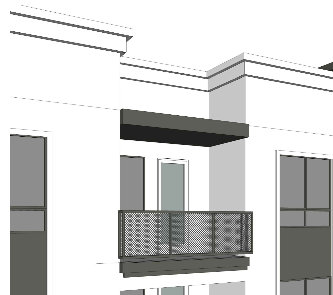
7. PAINTED 12" METAL AWNING AT DECK TO BE INSTALLED ± 9'-3" AFF
