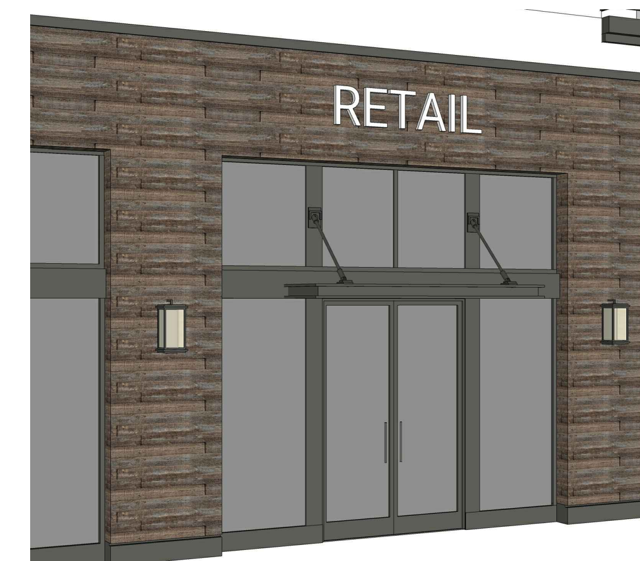
10. RETAIL STOREFRONT RECESSED 8" AT MASONRY VENEER W/ 8" BASE
