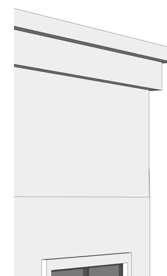
2. 8" X 18" PARAPET TRIM AT STUCCO MASSING
