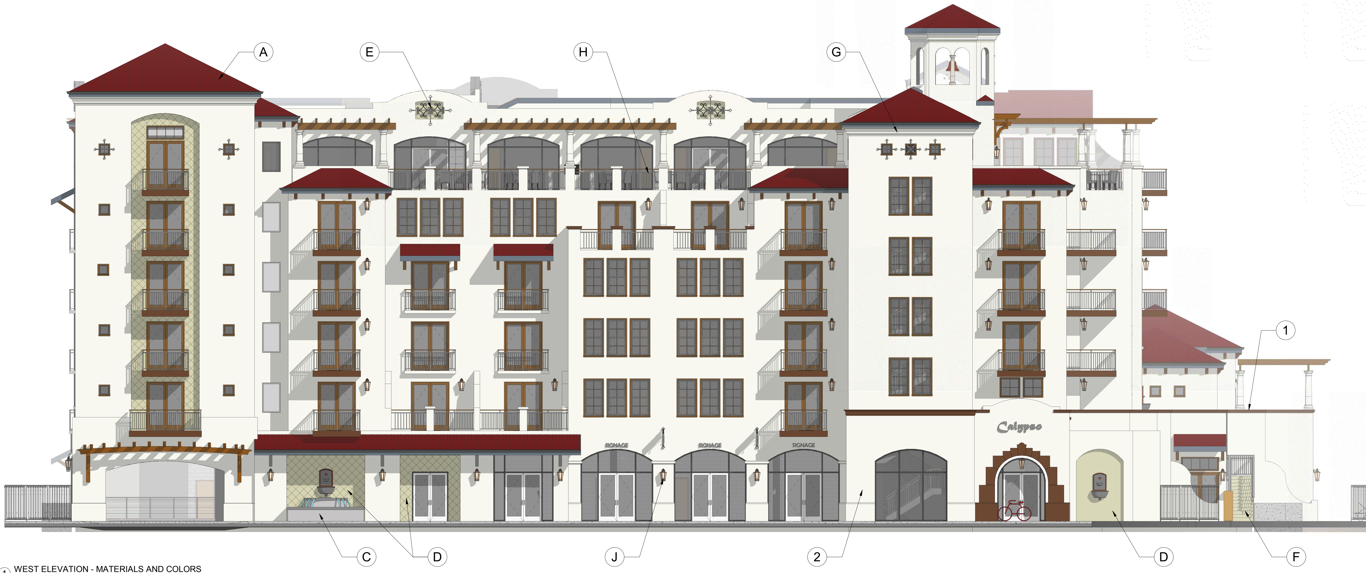
1 WEST ELEVATION - MATERIALS AND COLORS 1/8" = 1'-0"
