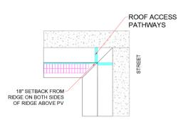
PV Less Than 33% Roof Area - Driveway Access (66% for homes with sprinkler systems)
