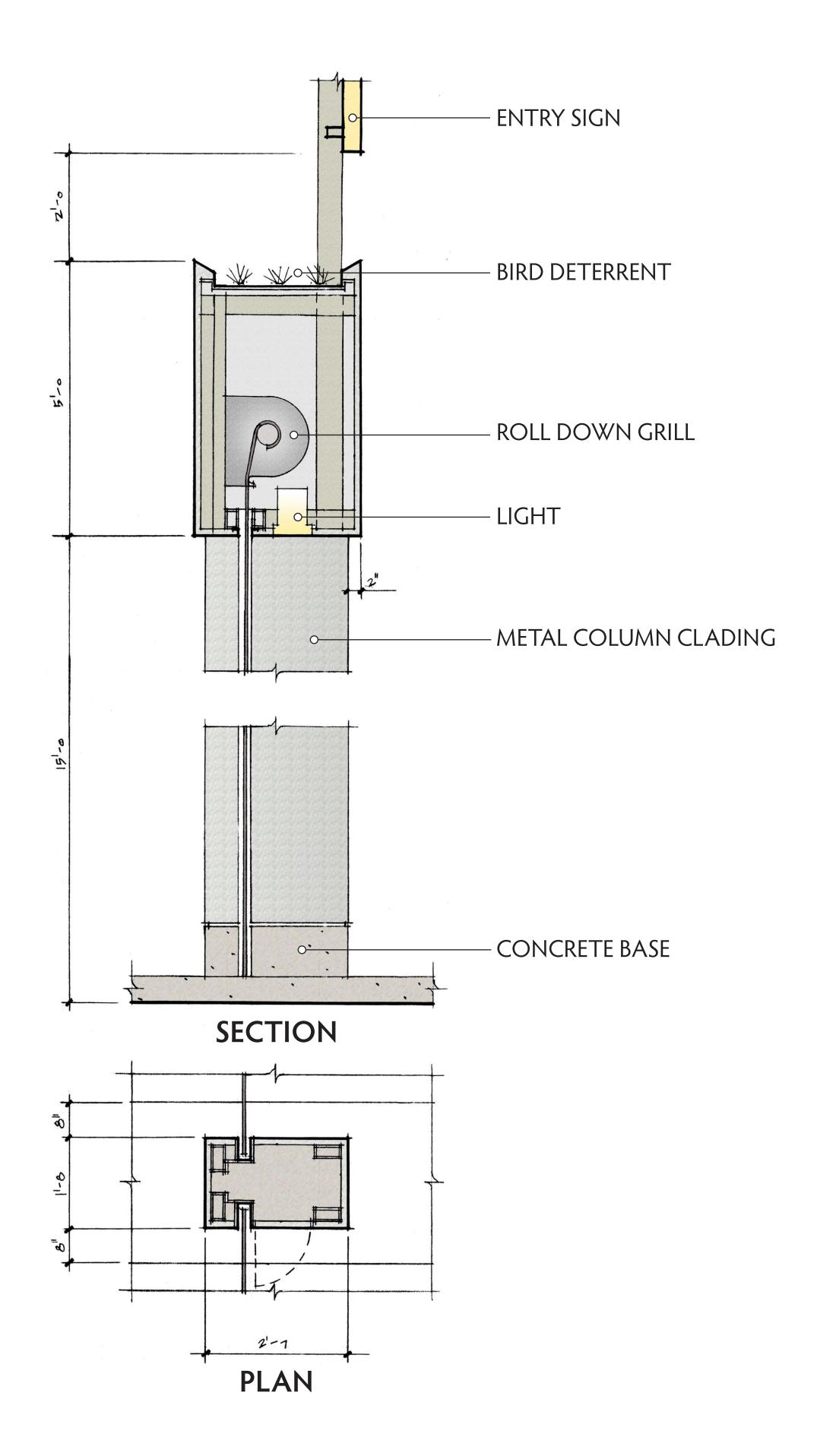
TYPICAL COLUMN OF THE ACCESS CONTROL MECHANISM AT PARKING GATES
